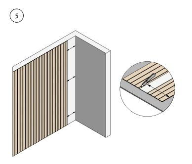
**5.** Before the last piece, measure the width between the panel and the wall in at least three different places to make sure the panel fits. Use the ThinRibbon ruler to draw a straight line and as a support when cutting the panel with our knife. Cut repeatedly times to achieve a neat cut.
