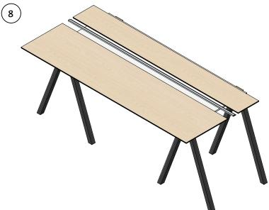
**8.** Loosely fit this together using our JOINT PROFILE.
