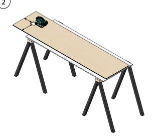
Transfer the measurements to the panel and saw out a hole using a compass saw.
