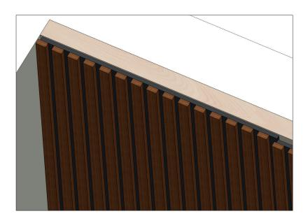
On one side of the panels goes one wooden slats over the edge. It is there to hide the joint.
