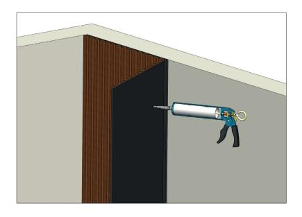
If you choose gluing, you get completely hidden mounting. Our fast-curing glue does it easy to glue the panels. Start always to glue on the panel.
